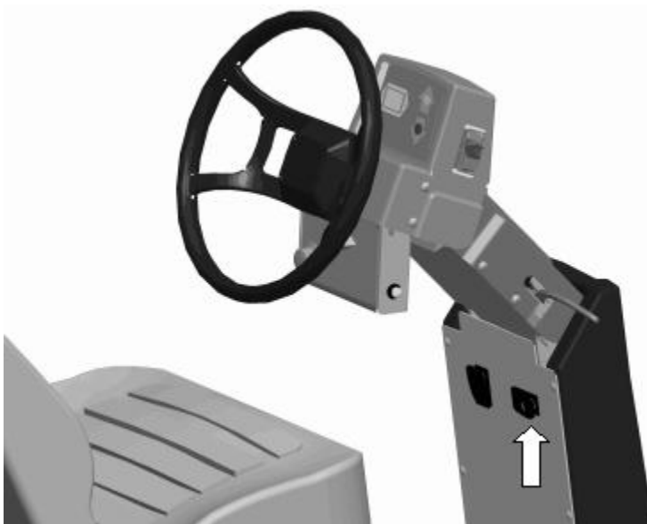
Location of Side Shift Switch
